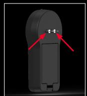
Check the pins to make sure they are screwed in tightly.
